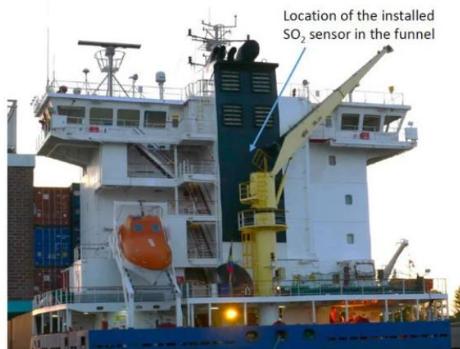
Figure 3. Container ship with approximate location of installed SO 2 sensors
