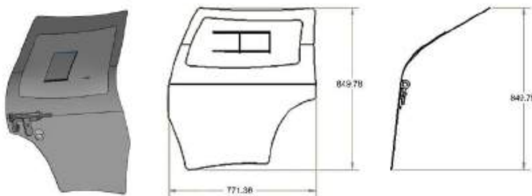
Figure 1. Car door design (unit in mm).
